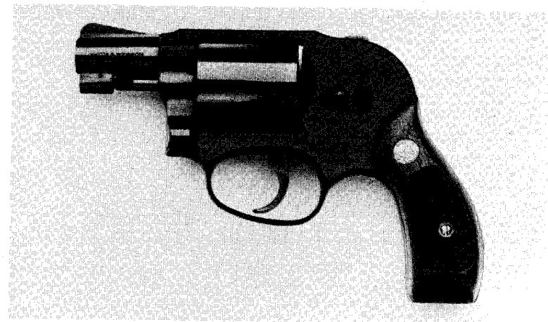
S&W MODEL 38 BODYGUARD: A 2-inch-barreled snubby that makes an excellent .38 Special pocket gun.
